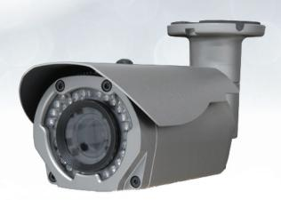
Vicon's V922 high definition (HD) vandal bullet camera is designed for security installations that need a compact vandal resistant camera that delivers outstanding imaging at 1080P. The motorized focus and zoom 5-51mm lens delivers high quality images for long range targets. In order to adapt to the low light lighting conditions, the V922B has integrated IR LEDs designed to illuminate the scene up to 25 meters.
