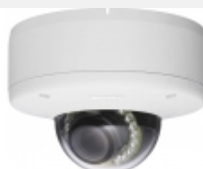
SNC-DH180 Outdoor IR Ruggedized 720p/30 fps Camera - V Series
