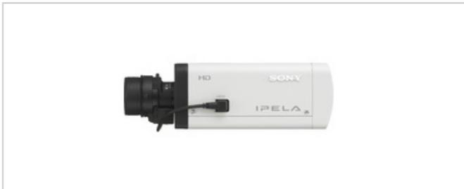
The SNC-CH120 is a high definition (720p) fixed network security camera with true Day/Night, Intelligent Motion Detection, DEPA analysis and is ONVIF compliant. It supports dual streaming of H.264, MPEG-4 and JPEG at full frame-rate.
