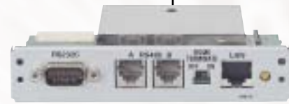
VZU-COM300 (sold separately). This is an optional communication board that provides LAN / RS-485 / RS-232C connection.
