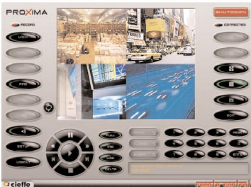
trolled in full or 1, 4, 9 or 16 way split screen. Currently supported PTZ camera protocols include: Sensormatic, Ultrak, Panasonic, Pelco, Samsung, Philips, Star Micronics, Kalatel, Vicon, JVC, Alec Dragon and others.
