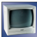
MV-120DS 12", high resolution monochrome monitor with audio
