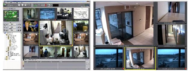
Although digital to its core, the Latitude can be either digital or analog at the edge. View live and recorded images on a PC monitor or an analog CCTV monitor. Control camera selection and PTZ camera control from a PC keyboard and mouse or from a traditional CCTV keyboard. Feed the system with IP networked cameras or traditional analog cameras. No matter the data source, analog or digital, the Latitude NVMS engine is 100% digital.
