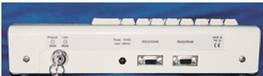
Rear panel of keyboard showing program switch, power jack and 2 RS485 / RS232 Ports.
