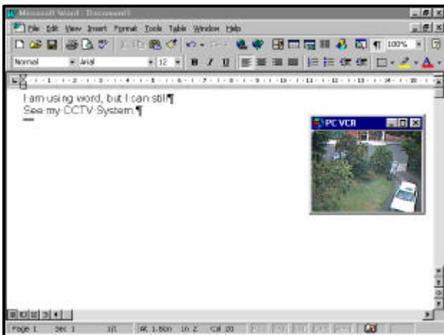
PC VCR enables you to constantly view images from the camera and records those images so that they can be found and replayed easily. PC VCR has the added advantage of being able to view stored images whilst still recording.
