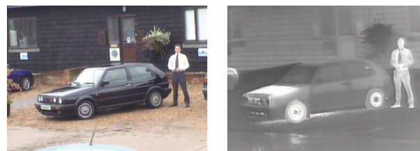
Optical image / Thermal image in white hot spot mode
