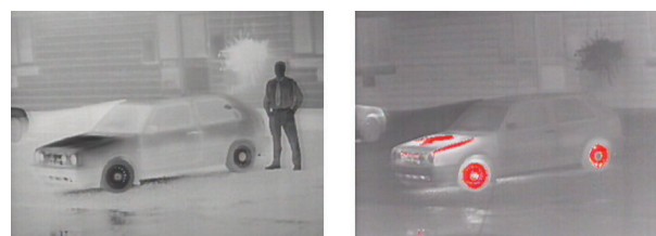
Thermal image in black hot spot mode / Thermal image in ice and fire mode
