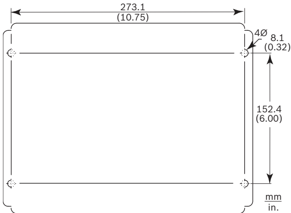
Mounting Hole Pattern
