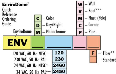
\* NOTE: No transformer included. Customer must supply 24 VAC, 50 VA transformer (LTC 5401 or equivalent). Not available with fiber optic option.
