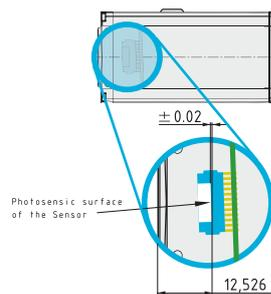
The back focal length on each camera is carefully measured and adjusted by our patented "CSAT" procedure. This guarantees an optimum distance between the lens flange and the sensor and ensures outstanding image quality based on compliance with optics standards.
