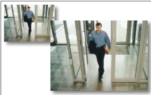
The increased resolution can also be used to provide a significantly larger overview. The inner rectangle below shows the area covered by an analog high-resolution camera. With the same number of pixels per area, the full 1280x1024 resolution provided by AXIS 211M - the outer rectangle below - covers a three times larger scene.
